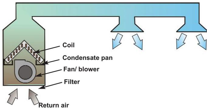
Return air from the house is filtered and blown through the air conditioner coil fins, which are chilled. The filtered return air is chilled by passing over, under and around the chilled aluminum fins and copper tubing.
