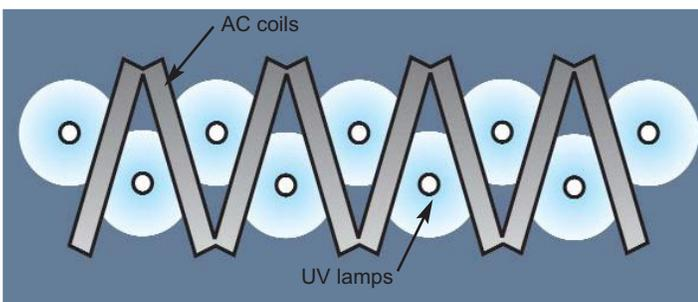
**Note of caution:** Unprotected UV-C lamps were used for this article. In practice, protected lamps should always be used as UV lamps contain mercury, a hazardous heavy metal known to cause health problems. A broken lamp in an HVAC system could permanently contaminate the system.
